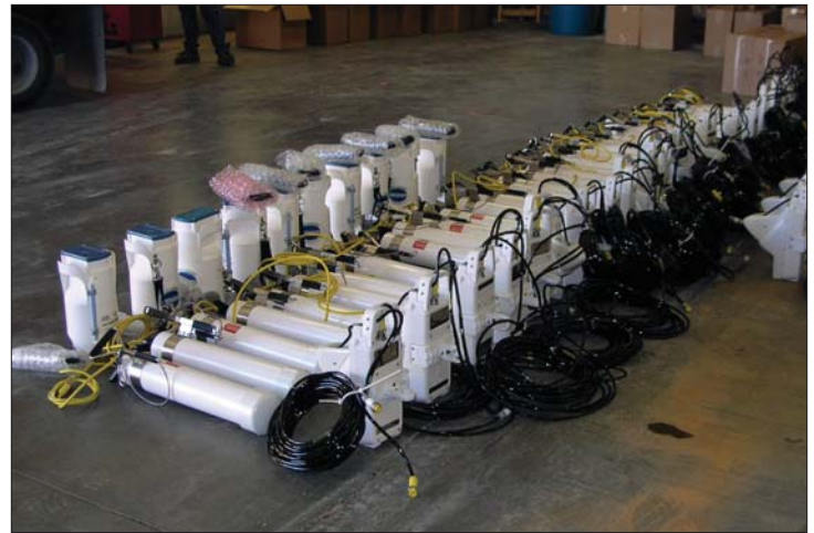
The program included the installation of 31 flow monitors and eight rain gauges from Marsh-McBirney/Hach.
